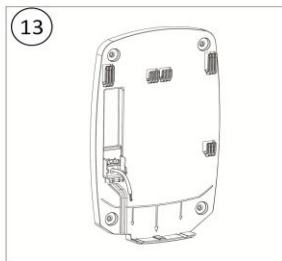
Route the wires through the Plug-in base as shown on the picture
