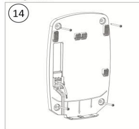
Screw the Plug-in base to the wall (x4)
