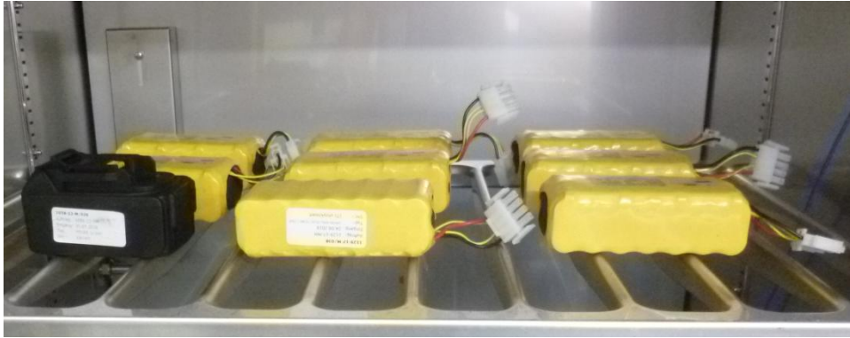
Figure 3: Thermal test in climate cabinet with the batteries inside
