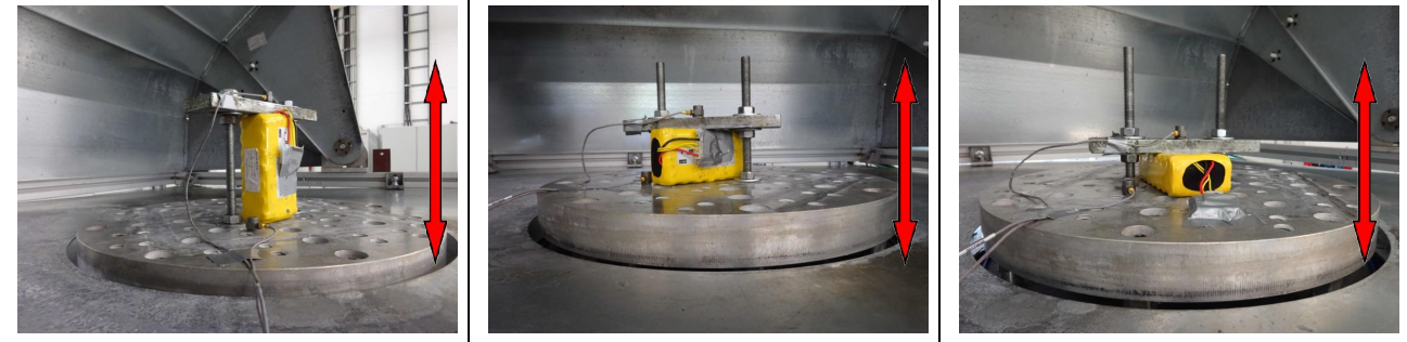
Figure 7: Shock test on shaker table with the batteries
