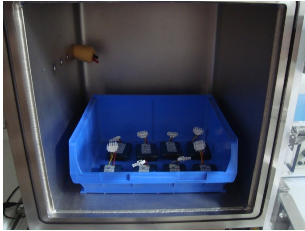
Figure 1: Pressure level in test chamber with the batteries inside
