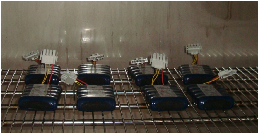
Figure 3: Thermal test in climate cabinet with the batteries inside
