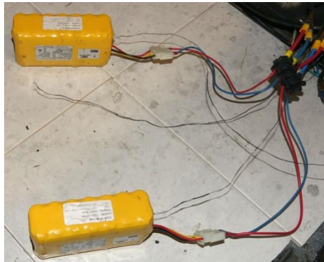
Figure 9: Short-circuit test in heat cabinet at 55 °C with the batteries
