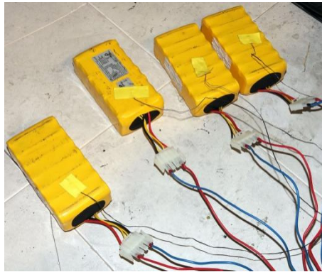
Figure 11: Overcharge test in safety cabinet with charge equipment (overcharge current 16 A, overcharge voltage 35.1 V)
