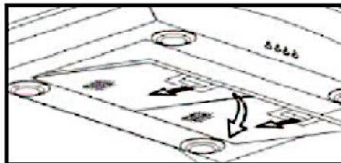
2. Soak the aluminium grease filter(s) in warm rinse water (up to 55 °C).
