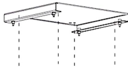
2. When having inserted the suitable fixing material (dowels, anchorages, etc.) into the ceiling and fixed it securely, screw the mounting plate tightly.
