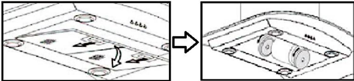
2. The CARBON FILTERS are intended to be installed on **both sides** of the motor (s. above; fig. on the right).
