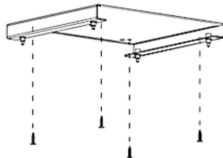
3. Connect the decor plate with the mounting plate using the appropriate screws: 2\*ST4 (8 mm).
