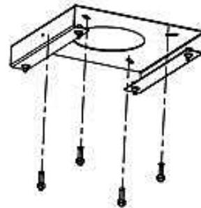
3. Connect the decor plate with the mounting plate using the appropriate screws: 2\*ST4 (8 mm).
