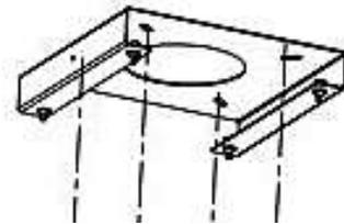
2. When having inserted the suitable fixing material (dowels, anchorages, etc.) into the ceiling and fixed it securely, screw the mounting plate tightly.
