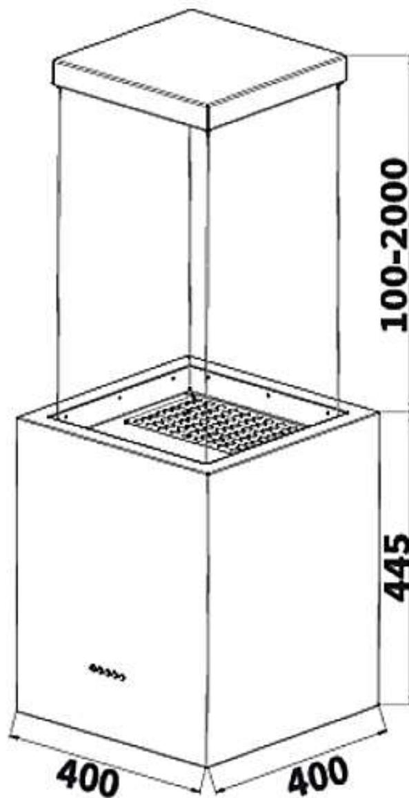
❏ Abmessungen in mm
