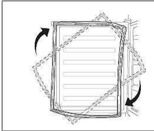
31. Open the doors of the appliance and reinstall the previously removed door trays / glass shelves / freezer drawers / etc.
