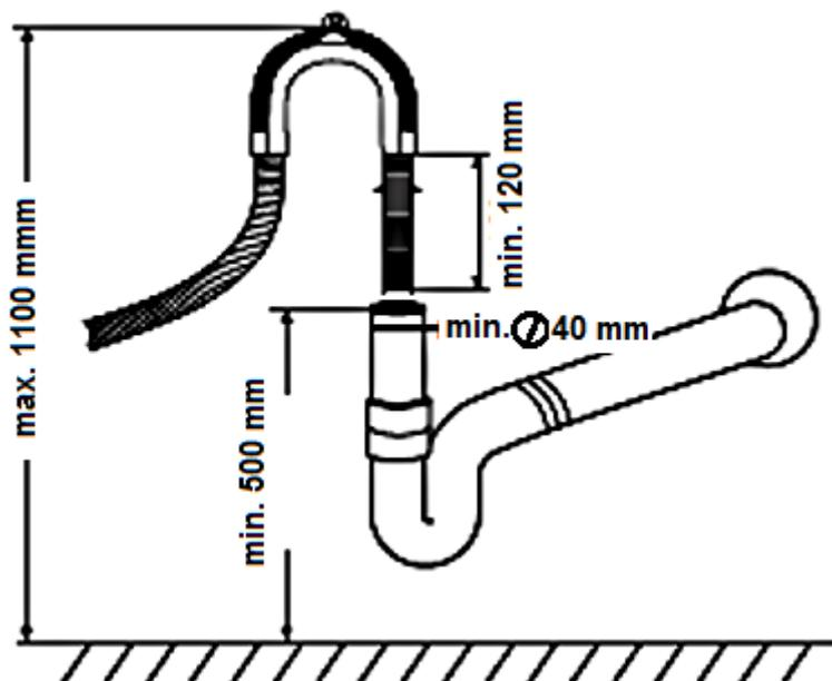
**Wastewater hook-up.** Fit the drainage hose of your appliance to the drainage pipe without bending. If the length of the hose is not sufficient, apply to your authorized service for an extension made from the same material as the original hose. Remember that the length of the hose (including extension) should not exceed 4 meters.
