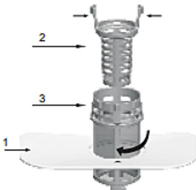
1. The **flat filter** catches remnants by a special nozzle on the bottom of the spray arm.
