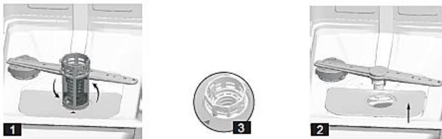
1. Turn the coarse filter anticlockwise and lift it up.
