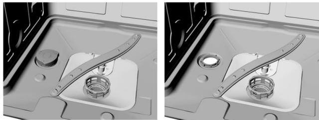
1. Remove the lower dish-rack and the lid of the water softener container.
