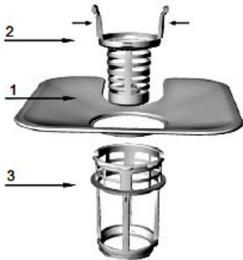
1. The **flat filter** catches remnants by a special nozzle on the bottom of the spray arm.
