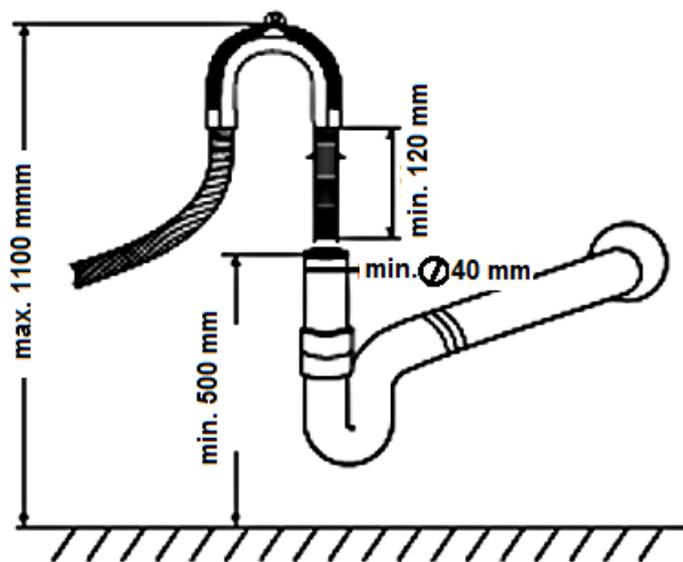
Fit the drainage hose of your appliance to the drainage pipe without bending.
