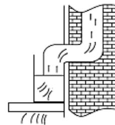
**HORIZONTALLY:** Lay the exhaust hose to an exhaust outlet equipped with an air grille\*.
